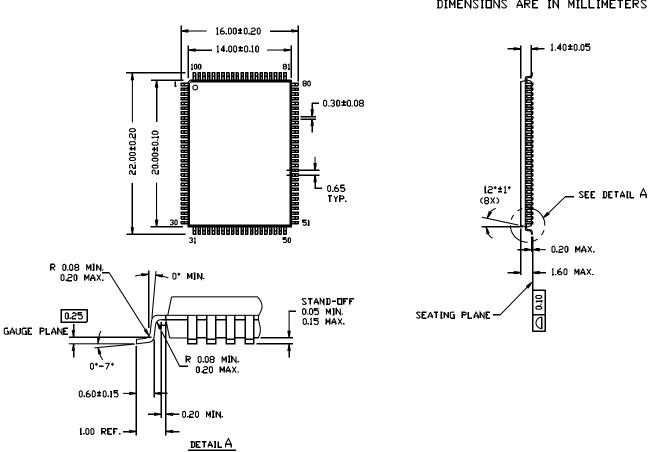
100-Pin Thin Plastic Quad Flatpack (14 x 20 x 1.4 mm) A101 DIMENSIONS ARE IN MILLIMETERS.
