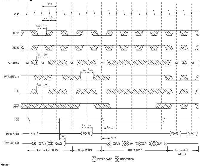
18. The data bus (Q) remains in high-Z following a WRITE cycle, unless a new read access is initiated by ADSP or ADSC 19. GW is HIGH.
